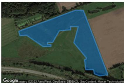
**Name:** PV Feld 3**Footprint area:** 28,919 m<sup>2</sup>**Axis tracking:** Fixed (no rotation)**Tilt:** 10.0 deg**Orientation:** 180.0 deg**Rated power:** -**Panel material:** Smooth glass with AR coating**Vary reflectivity with sun position?** Yes**Correlate slope error with surface type?** Yes**Slope error:** 8.43 mrad
